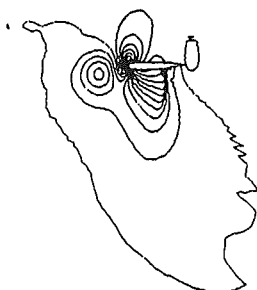
Fig. 11(a) Pressure contours ( t = 4.5 )
